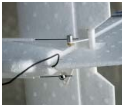
High quality "keeper" style connectors hook the pushrods to the elevator and rudder horns.
