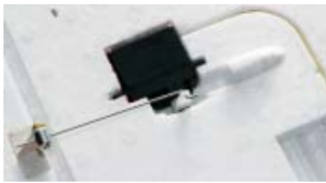
The right aileron servo is shown nested in the aileron bay. I wrap black electrical tape around the servo (with the end of the tape concealed under the servo) and CA the taped section to the foam to simplify removal.
