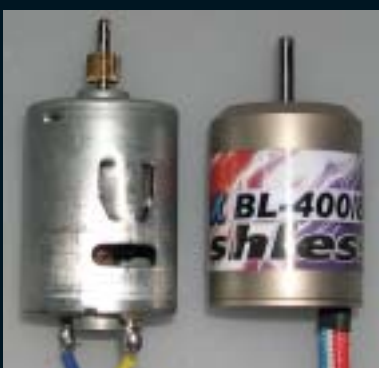
The stock Permax 400 brushed motor (left) and the new 400 brushless motor. The hop-up motor will drop into the same gearbox using special pinion and spur gears.
