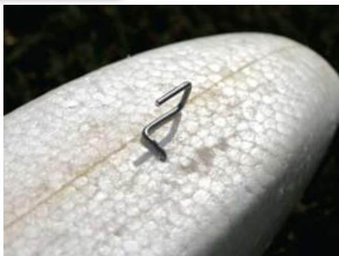
▲ Here is a close-up photo of the custom-bent hook for the nose of the Easy Glider. Simply push it into the foam and tape in place with high-strength tape.
