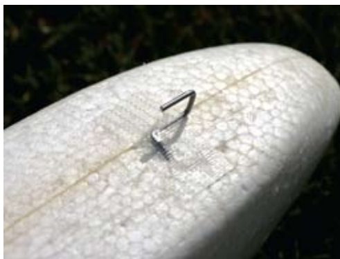
▲ Here is a close-up photo of the custom-bent hook for the nose of the Easy Glider. Simply push it into the foam and tape in place with high-strength tape.
