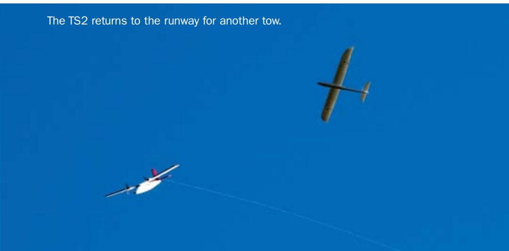
At the point of release, the TS2 slows down and the Easy Glider slips off the line.
