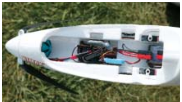
The canopy functions as a large access hatch that snaps down over all the equipment. The battery sits right on the CG, so you could use batteries in a variety of sizes without having to re-trim.
