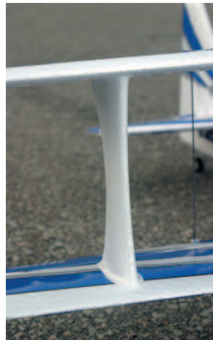
The airfoil-shaped I-struts are glued to the top and bottom wing. The wing assembly is removable from the fuselage.
