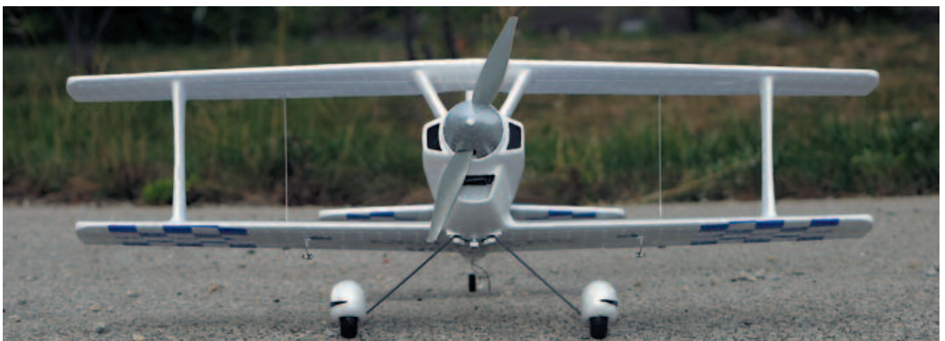
The Elapor construction is rugged. Even the spinner is made from the material, which was painted silver with Rust-Oleum spray.
