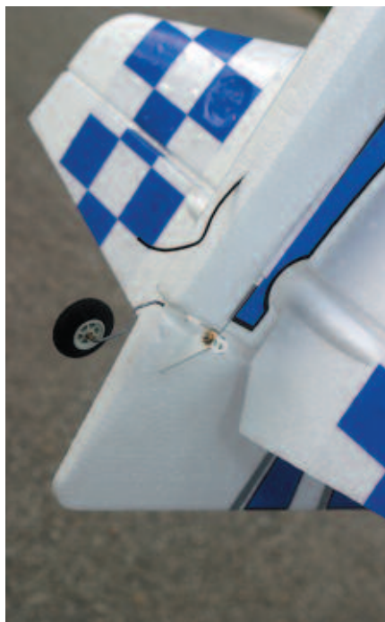
The assembly process can be finished more quickly because the hinges are molded into the control surfaces.
