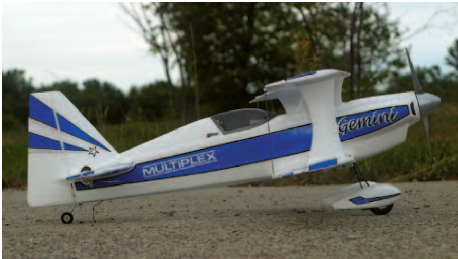
A profile view shows the built-in thrust and incidence angles. Fuselage decals hide the elevator and rudder servos as well as the pushrods. Motor thrust is adjustable.
