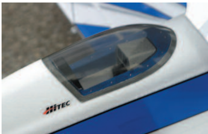
The builder can choose to paint the inside of the cockpit before attaching the tinted canopy with cyanoacrylate glue.
