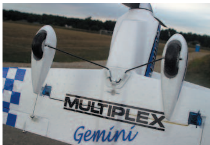
Hitec HS-55 servos complement the control surfaces. They fit perfectly inside the molded pockets and are held in with hot glue.
