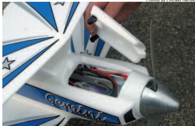
The front hatch encloses the 3S 2500 mAh Multiplex Li-Poly battery, which should be located as far forward as possible.
